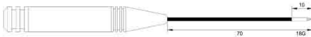
Fig. 1 Modified internally cooled electrode for thyroid lesion, which is shorter (7 cm shaft length) and thinner (18G) than conventional electrode
